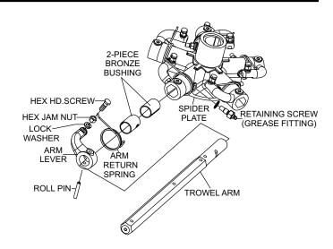
Figure 38. Trowel Arm Removal (Spider Plate)
